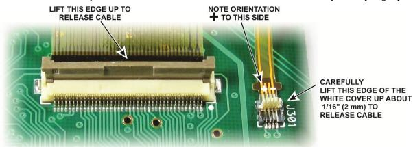
Figure 45. LCD Cable Connectors Opened.
