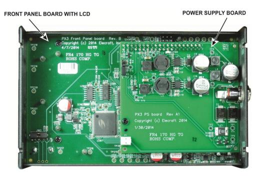
Figure 23 Assembled PX3 with Bottom Cover Removed.
