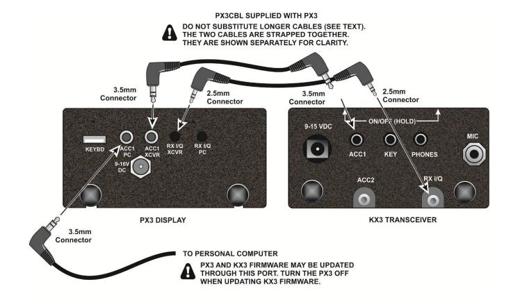
Figure 2. Basic KX3-PX3 Cabling.
