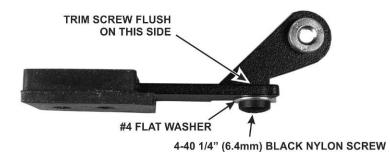
Figure 39. Placing Nylon Bumpers on the Tilt Legs.
