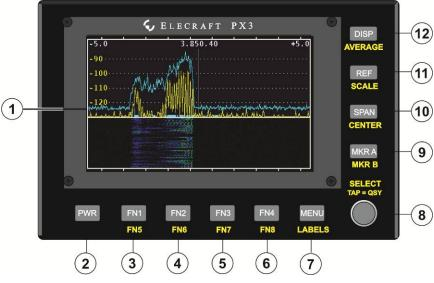
Figure 1. PX3 Front Panel.
