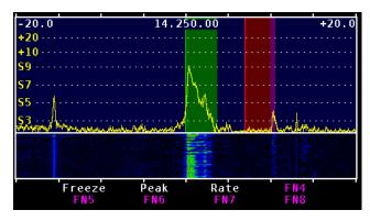
Figure 12. Red Bar Cursor Showing Transmit Frequency Above the Receive Frequency.
