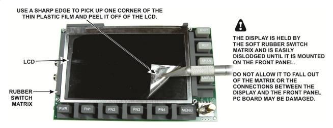
Figure 28. Removing the Plastic Film from the LCD.
