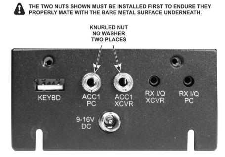
Figure 35. Mounting the Left Side Panel Part 1.
