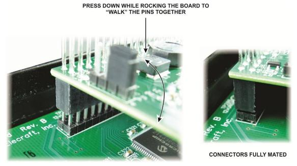
Figure 33. Mating the Power Supply Board Connectors.
