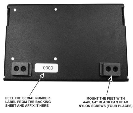
Figure 41. Installing Fixed Feet and Serial Number on Bottom Cover.
