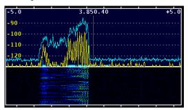
Figure 16. Typical SSB Spectra using Peak Hold.
