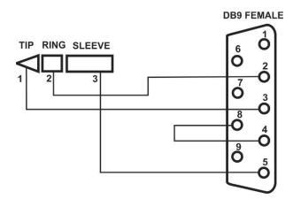
Figure 22. RS-232 Cable Schematic Diagram.
