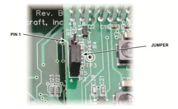
Figure 17. Power Control Jumper.
