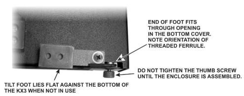
Figure 42. Installing the Tilt Feet in the Rear Cover.
