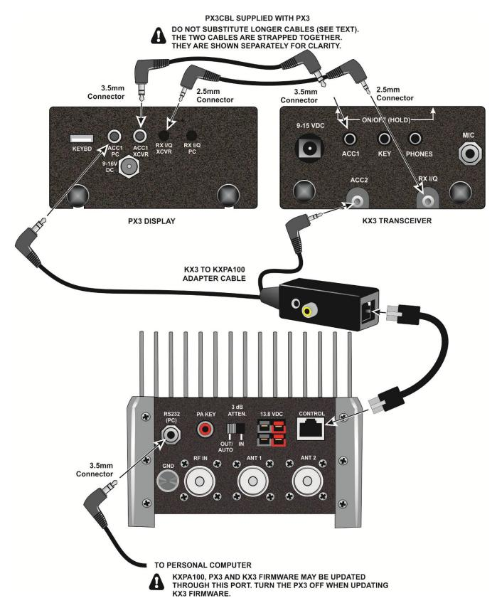
Figure 3. PX3 Signal Cabling with KXPA100 Amplifier and KX3 to KXPA100 Adapter Cable.
