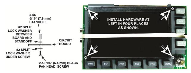
Figure 24. Mounting the Front Panel Standoffs.
