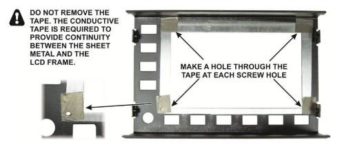
Figure 25. Front Panel Conductive Tape.
