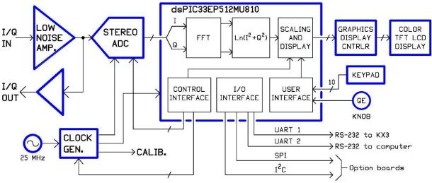
Figure 21. PX3 Simplified Block Diagram.
