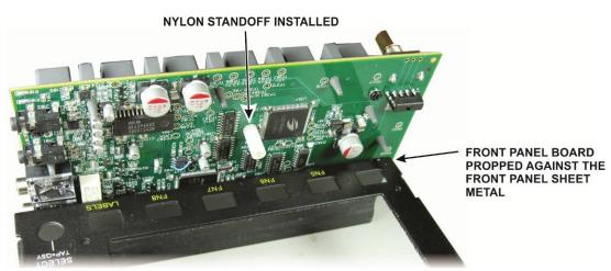
Figure 27. Nylon Standoff Installed.
