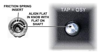
Figure 31. Installing the Knob.
